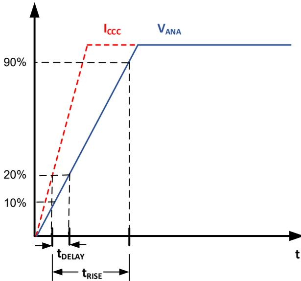
Figure 44. CT431 Propagation Delay and Rise Time Curve
