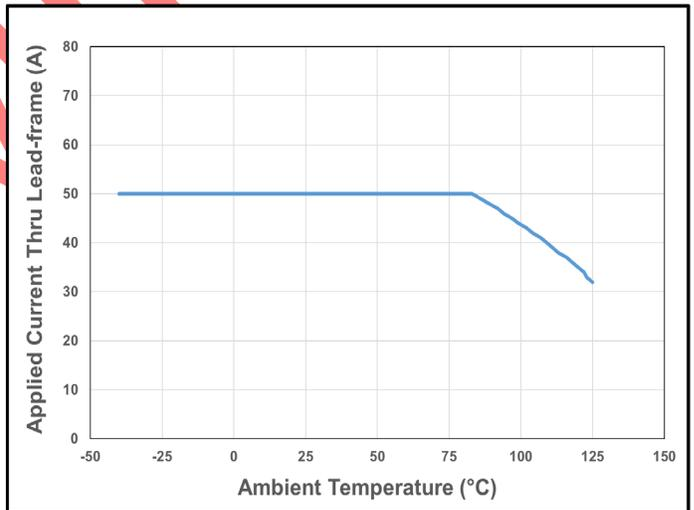
**Figure 36. CT431 Current De-rating Curve for 50 A<sub>DC</sub>**
