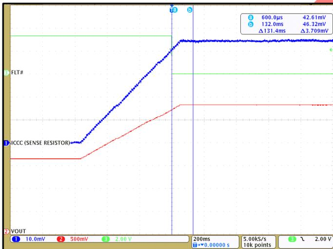
Figure 13. CT431 OCD enabled at +110% of +50 A<sub>PK</sub> and FLT# is LOW
