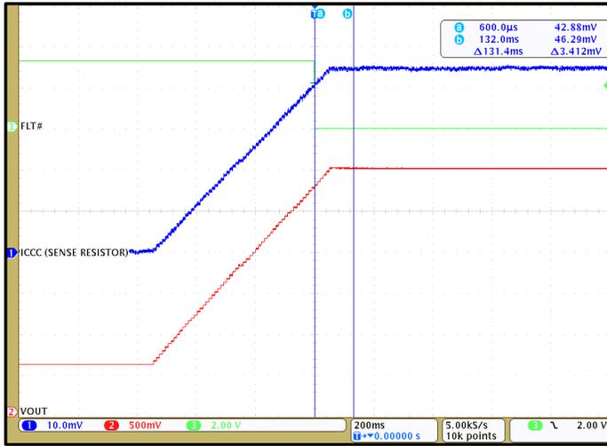
Figure 11. CT431 OCD enabled at 110% of +50 A<sub>DC</sub> and FLT# is LOW
