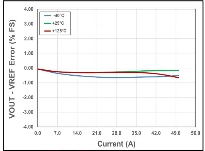
**Figure 34. VOUT - VREF Error vs. Current vs. Temperature**
