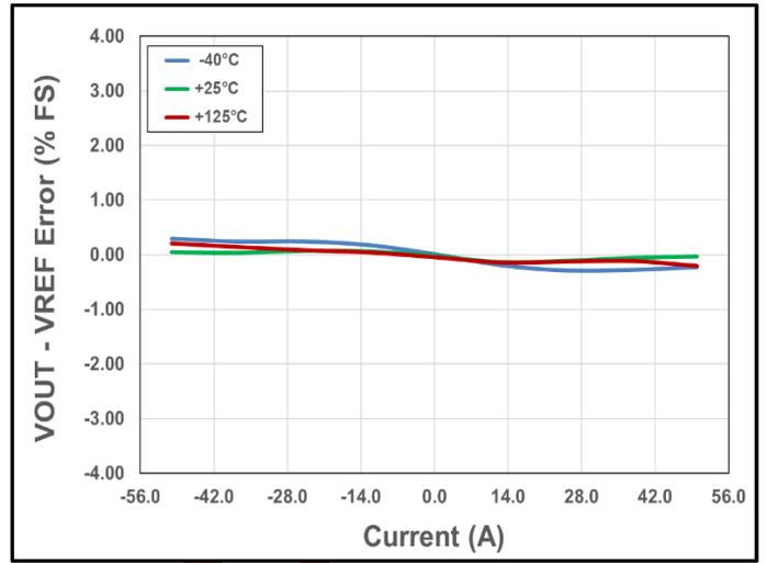
**Figure 38. VOUT - VREF Error vs. Current vs. Temperature**
