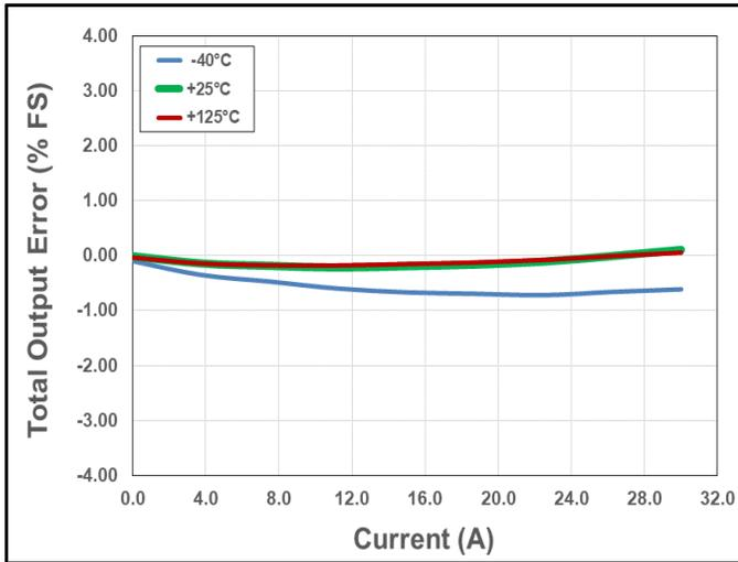
**Figure 25. Total Output Error vs. Current vs. Temperature**
