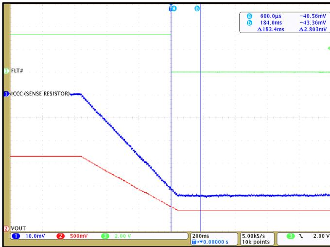
Figure 15. CT431 OCD enabled at -110% of -50 A<sub>PK</sub> and FLT# is LOW
