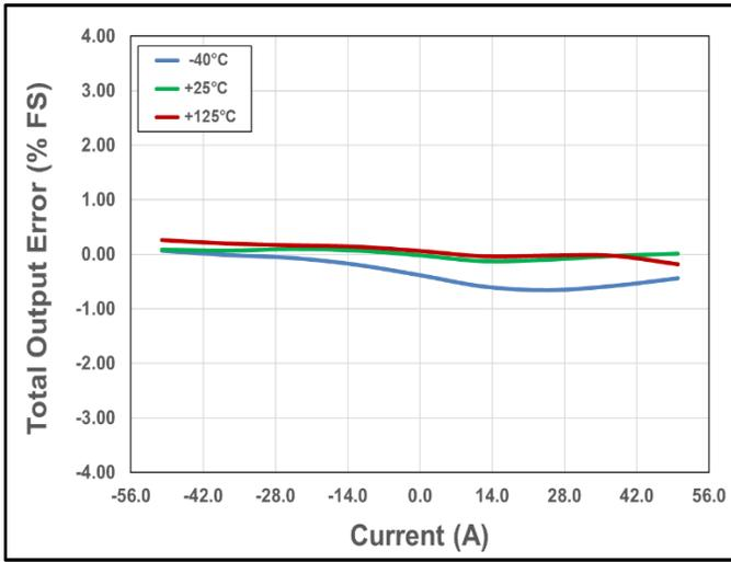
**Figure 37. Total Output Error vs. Current vs. Temperature**
