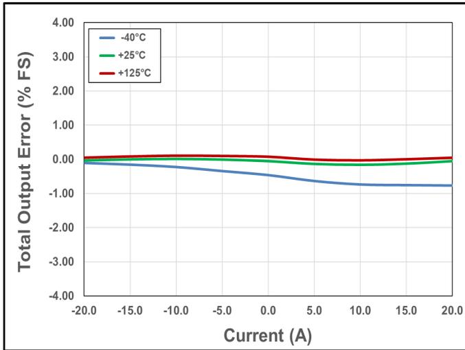
Figure 21. Total Output Error vs. Current vs. Temperature
