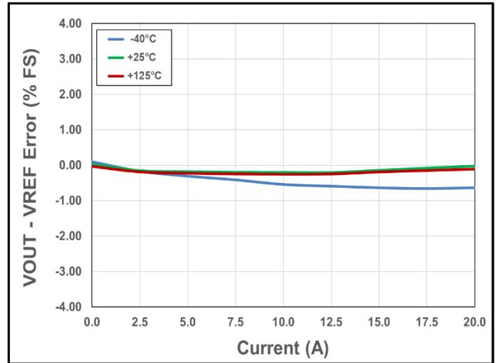
Figure 18. VOUT – VREF Error vs. Current vs. Temperature
