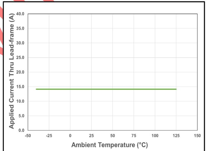
Figure 24. CT431 Current De-rating Curve for 20 A<sub>PK</sub> (14.1 A<sub>DC</sub>)
