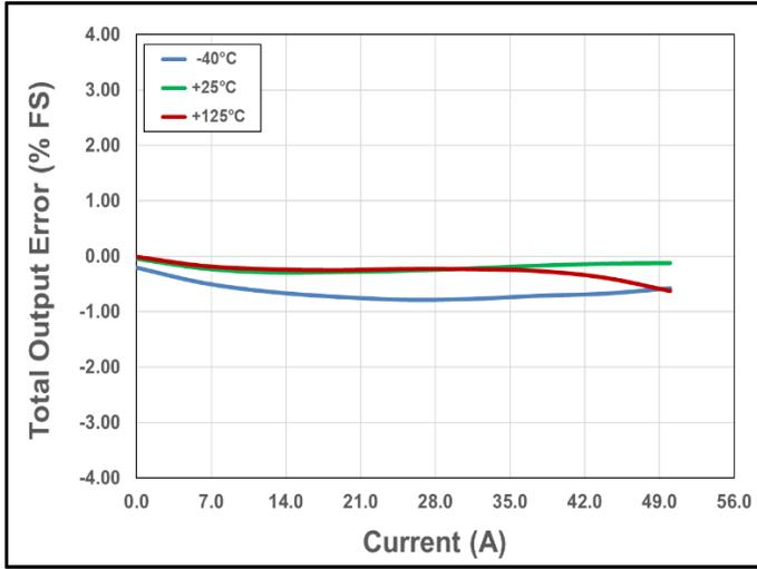
**Figure 33. Total Output Error vs. Current vs. Temperature**
