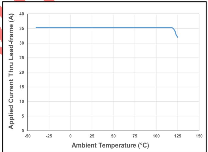
**Figure 40. CT431 Current De-rating Curve for 50 A<sub>PK</sub> (35.4 A<sub>DC</sub>)**
