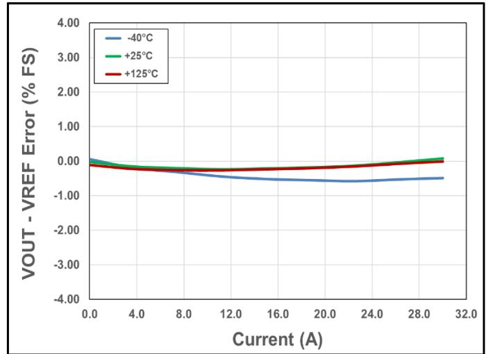
**Figure 26. VOUT - VREF Error vs. Current vs. Temperature**
