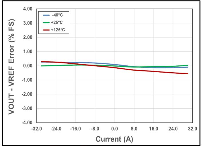
Figure 30. VOUT - VREF Error vs. Current vs. Temperature
