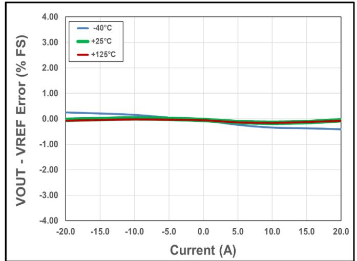
Figure 22. VOUT - VREF Error vs. Current vs. Temperature
