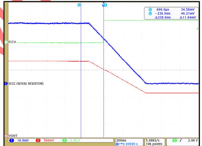
Figure 14. CT431 OCD disabled at +90% of +50 A<sub>PK</sub> and FLT# is HIGH
