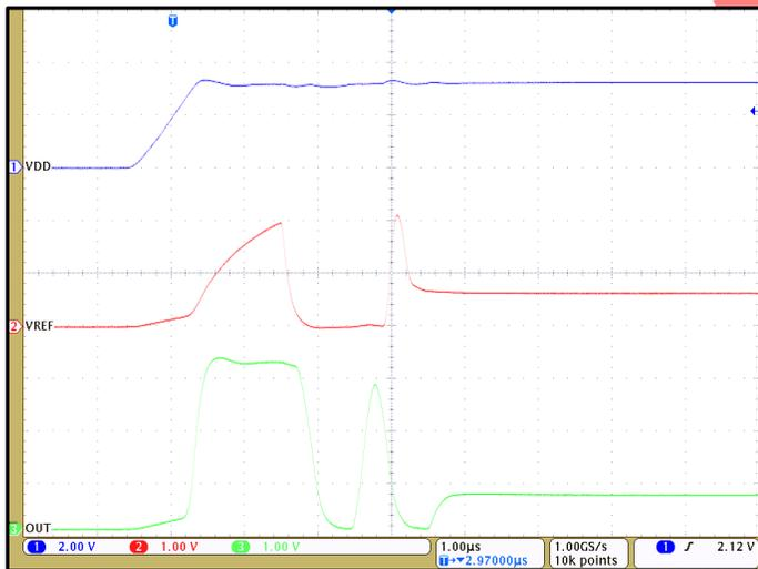
Figure 5. CT431 Startup Waveforms for  $V_{OQ} = 0.65\text{ V}$
