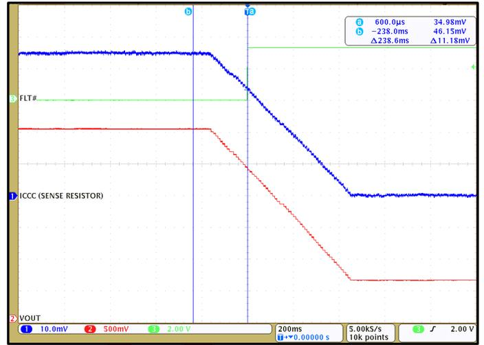
Figure 12. CT431 OCD disabled at 90% of +50 A<sub>DC</sub> and FLT# is HIGH
