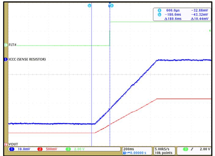
Figure 16. CT431 OCD disabled at -90% of -50 A<sub>PK</sub> and FLT# is HIGH
