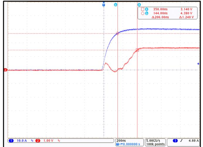
Figure 8. CT431 Response Time; I<sub>P</sub> = 30 A<sub>PK</sub> and C<sub>L</sub> = 220 pF
